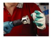
Remove tile debris from the drill bit.
